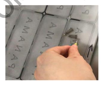
② loose the injection gun cap to put pin on injection gun and cover the cap and tighten. parallel injection guns install same size pin .
